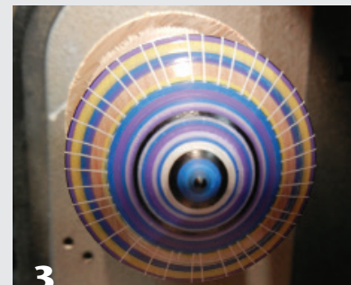
3 Centrifugal force will “throw” the paint outward from its point of application.
