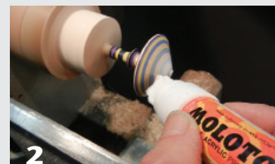
2 Use high-flow paint in a pen or marker to add the “splash” effect.
