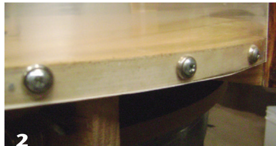
2 The top is mounted onto rails, which are inset from the edge. The Plexiglas is screwed to the edge of the arena.
