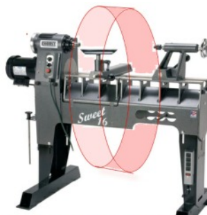
Avoid the Danger Zone When Starting Your Lathe
