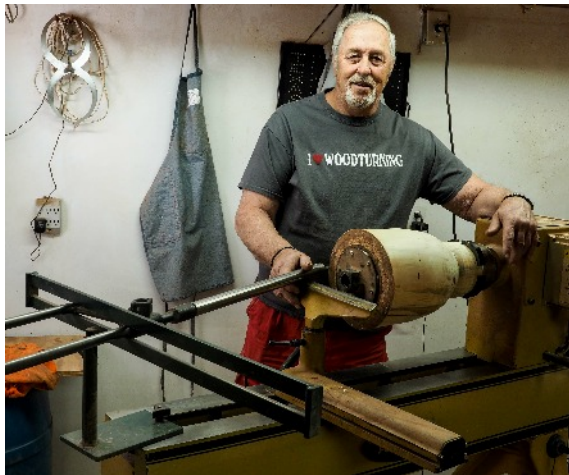
Randy in his shop showing his boring bar on the Powermatic lathe (his third lathe).
