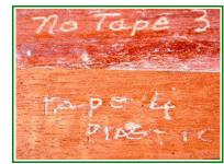
In the image at left plastic tape was applied to the portion lower of surface, leaving the upper surface clear. The plastic chosen for stickiness was so sticky that some liming was came away with the tape. In this view the No Tape 3 ap-
