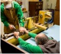
axis of the lathe. Turn ends to round watching shadow on back side of ball. Rotate the ball 90 degrees and continue to round visualizing shadow. Repeat until shadow can no longer be seen.
