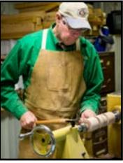
The November demonstration was done by Larry Rogers. Larry reprised a demo from 2008 or 2009. Larry's sphere making technique is an Old World method. A billet is turned to a cylinder whose diameter equals the sphere's desired size. Using a caliper, the diameter is scribed onto the cylinder.
