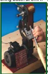
Proedge sharpening system. Without AAW this purchase would not have been possible. Other uses of the EOG has been an buying an additional lathe which may be seen in pictures on page 4 in the article on the latest beginner class.
