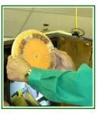
into rings. A jig constructed from HDPE or neoprene, the device holds segments of equal length in a common radius as shown in picture at left.
