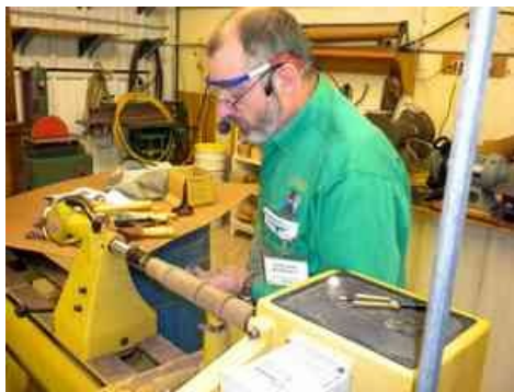
Marking reference points with parting tool
