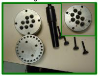
At far left are the base and face plates. The inset to the right shows the opposite side of the base plate, showing the numbered options for eccentric centers. The four knurled screws attach the face and base plates to each other. The iig is sold with optional hex screws. These
